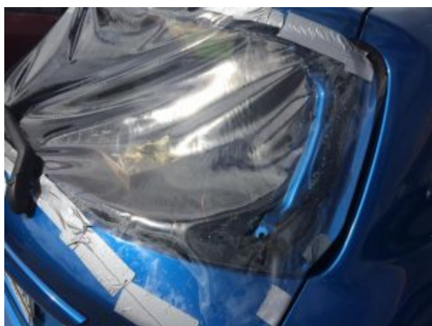
Plastic sheet attached with duct tape over the rear window to keep the rain out.
