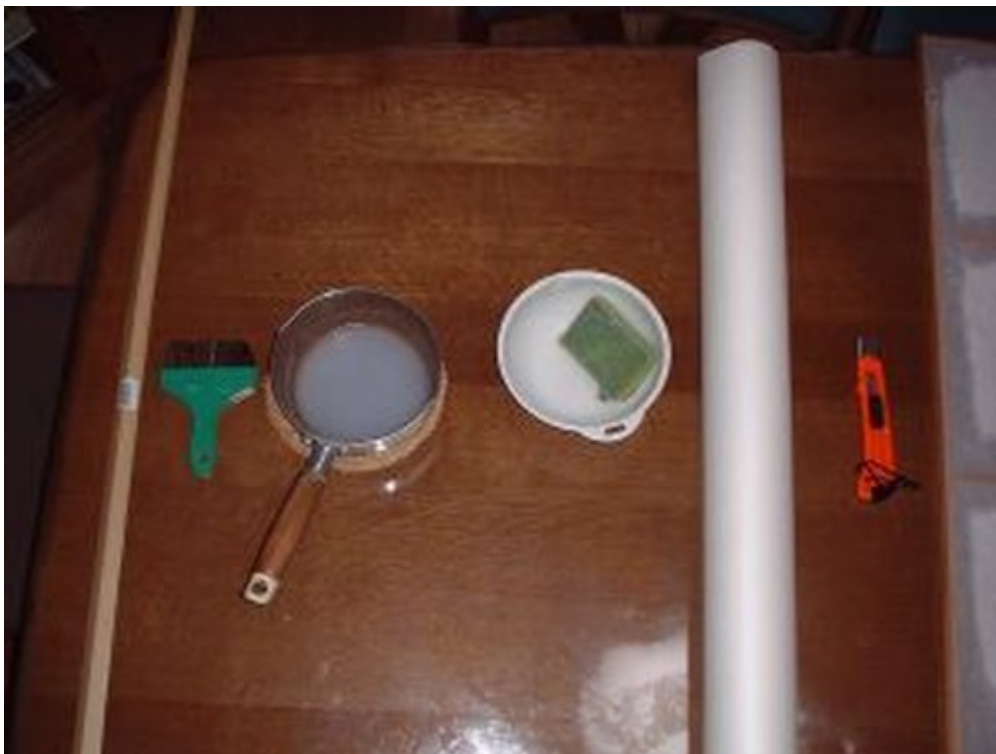
Materials needs to fix shoji doors
